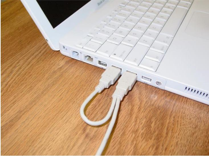
2. Plug the CDU-680 USB modem into the other end of the Y-cable:
